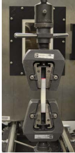
Figure 4. Tensile testing on Instron 5866 Mechanical Testing Machine.
