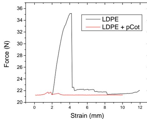
**Figure 5.** Strain curve of the virgin LDPE compared to the strain curve of LDPE with pCot.
