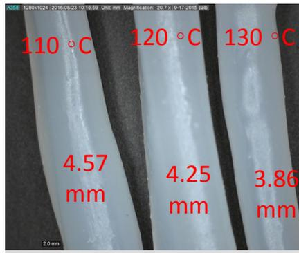
**Figure 1.** Comparison of LDPE filament extruded at temperatures ranging from 100-130 °C in a Noztek pro HT.
