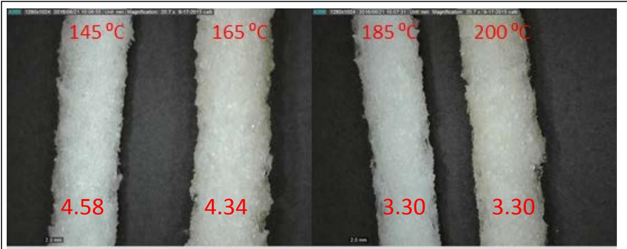
**Figure 2.** Comparison of the LDPE filament with 25 wt% pulverized cotton (pCOT) extruded at a temperature range of 145-200 °C in a Noztek pro HT.
