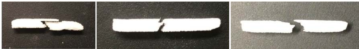
Fig. 10. Fractured silica beams post three-point bending test
