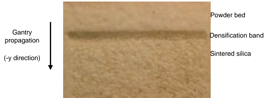
Fig. 4. Densification band in the powder bed
