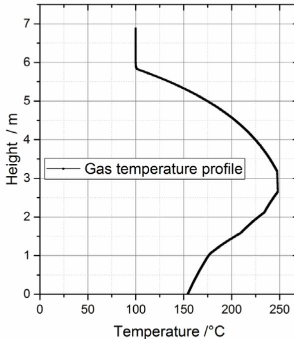
Figure 2: Temperature profile used for rounding of PBT-glass comminution products.
