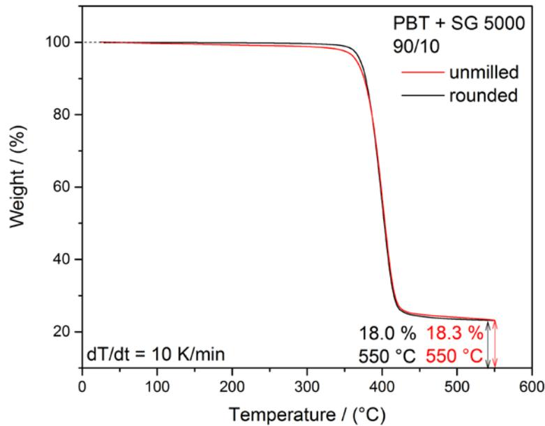
Figure 6: TGA curve of PBT+SG 5000 in a ratio 90/10 of the unmilled and rounded state.
