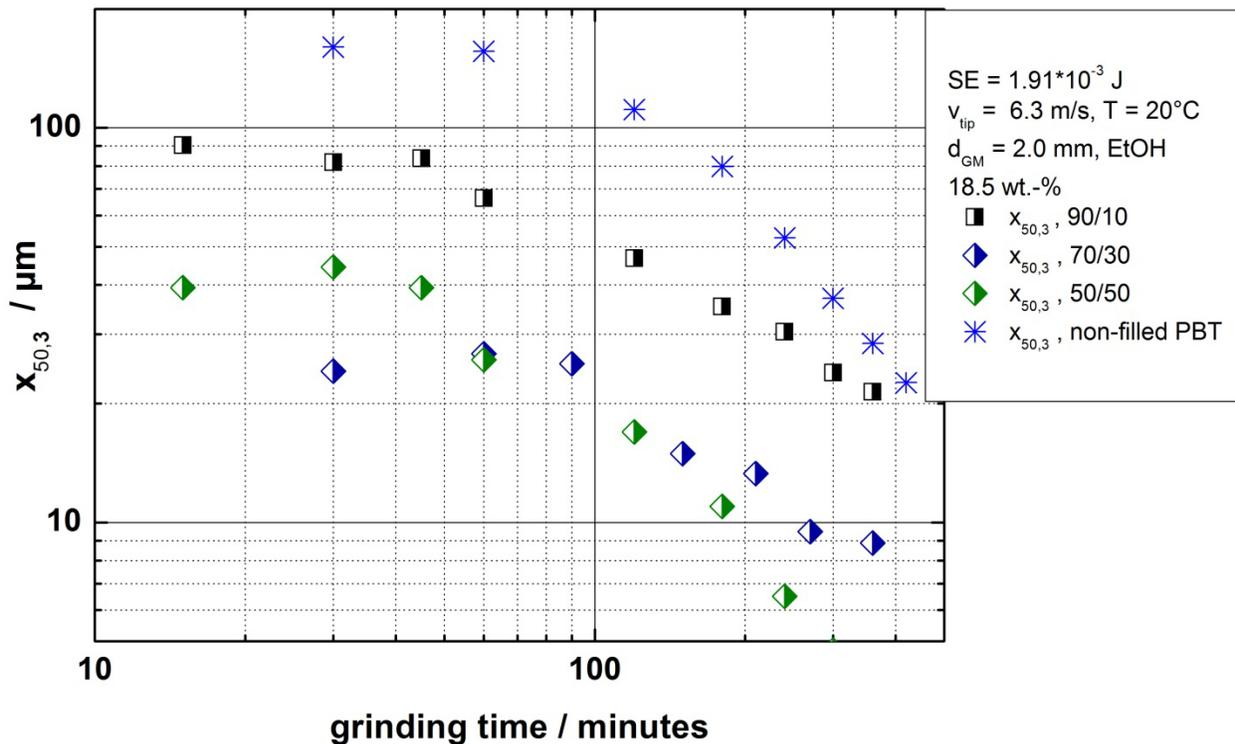
Figure 1: Evolution of product particle size  $x_{50,3}$  during wet grinding of PBT-glass (SG3000) composite material in ethanol: influence of polymer-to-filler volume ratio on grinding kinetics.
