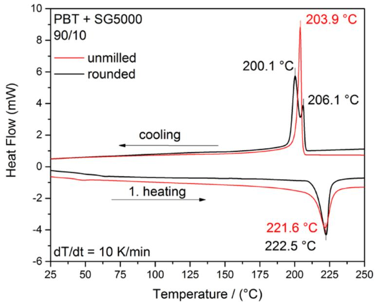
Figure 4: DSC curve of the first heating and cooling run of PBT+SG5000 in a ratio of 90/10 in the unground and rounded state.
