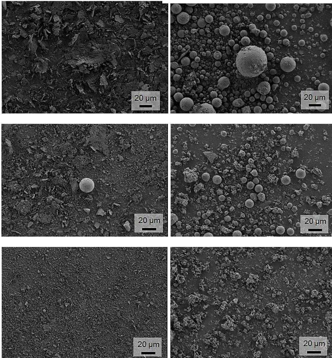
Figure 3: SEM images of the comminuted (left) and rounded (right) PBT-glass composite powders: 90/10 (top), 70/30 (middle), 50/50 (bottom).
