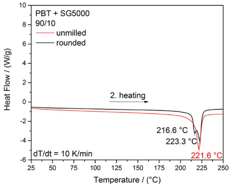
Figure 5: DSC curve of the second heating run of PBT+SG 5000 in a ratio of 90/10 in the unground and rounded state.
