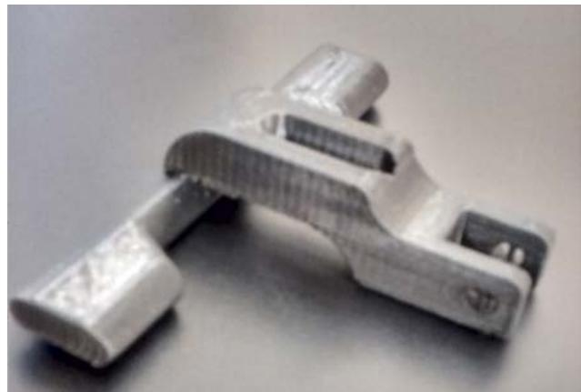
Figure 6: Actual part made on Makerbot
