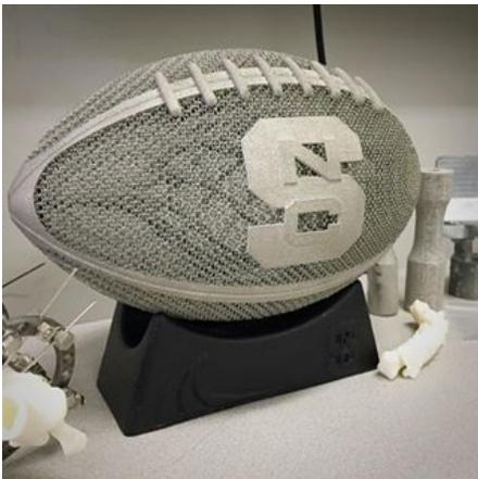
Figure 12: Porous Mesh Football built on the ARCAM EBM machine
