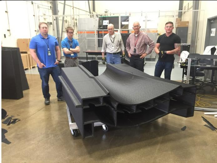
**Figure 3: Section of a wind turbine mold**
