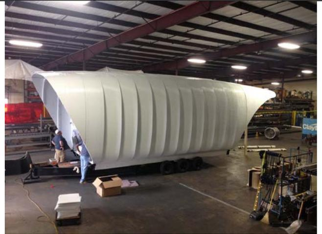
**Figure 4: Printed prototype house**
