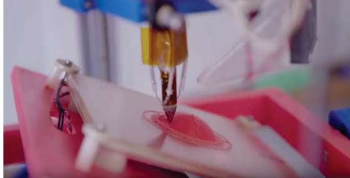
Figure 6: 5AAM machine in operation, showing coordinated motion of all five axes including local control of the nozzle perpendicular.
