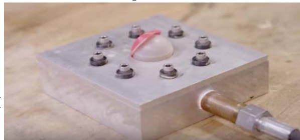
Figure 7: Typical failure mode of a hemispherical dome.
