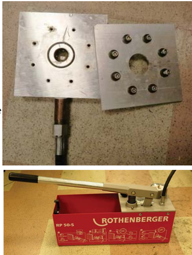
Figure 1: Pressure testing jig (above) and hydrostatic pressure testing pump (below)
