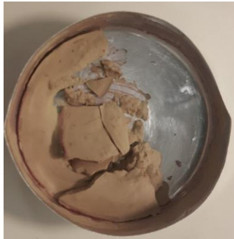
Figure 3. ECPC made of beeswax and silver coated nickel powder.
