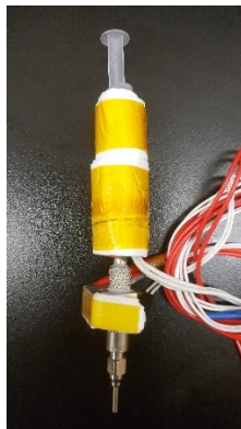
Figure 9. Molten solder extrusion.
