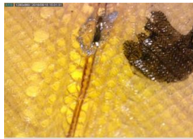
Figure 12. Solder paste-based junction reflowed by soldering iron.
