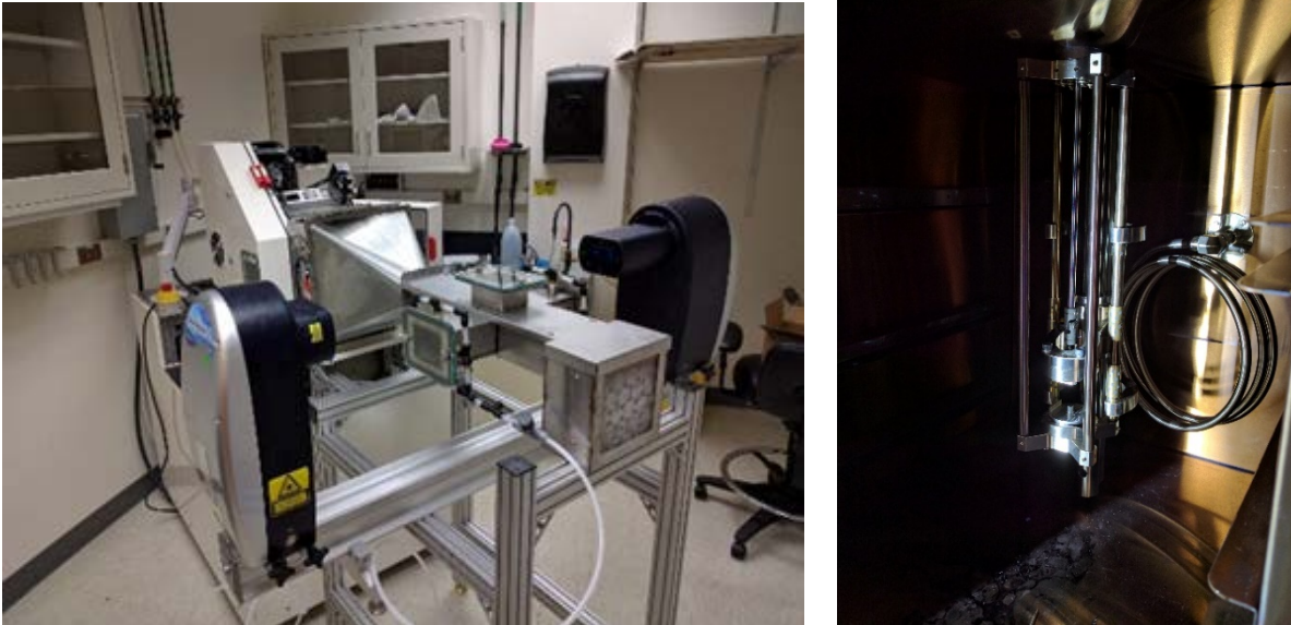
Figure 3 PARC's infrastructure for studying spray and extensional rheology. Left a complete spray system for experimental work and right an extensional rheology device mounted inside of an oven.
