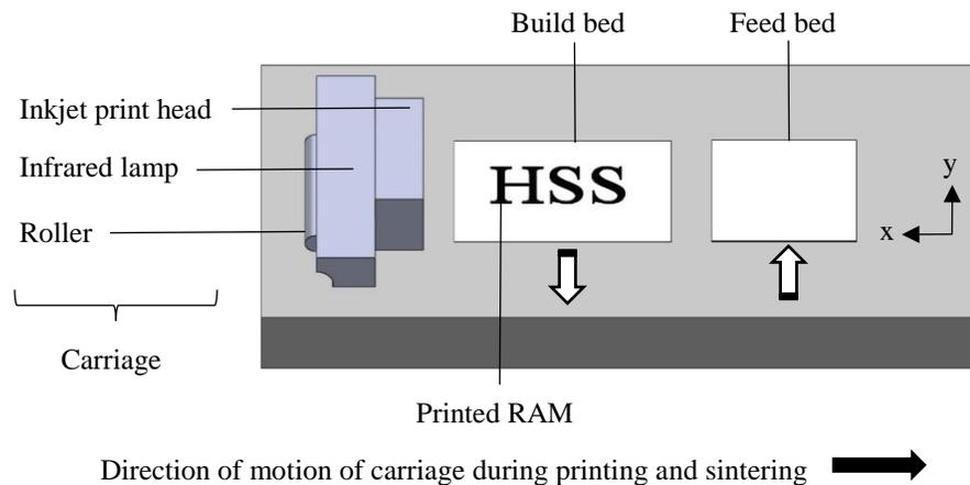
Figure 1: High speed sintering process
