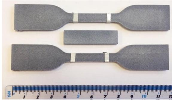
Figure 2: High speed sintered parts
