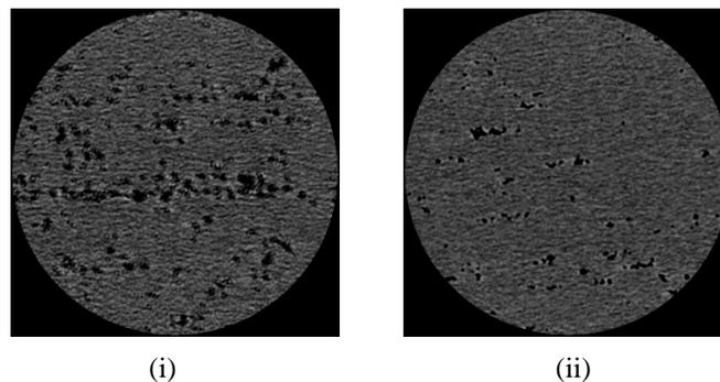
Figure 8: Cross-sectional images of high speed sintered parts manufactured by (i) Lamp 1 and (ii) Lamp 2
