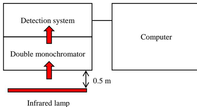
Figure 3: Plan view of irradiance measurement setup
