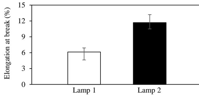
Figure 7: Elongation at break of high speed sintered parts
