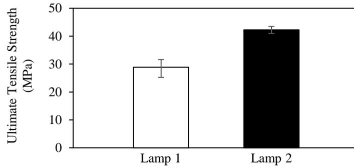
Figure 5: Ultimate tensile strength of high speed sintered parts
