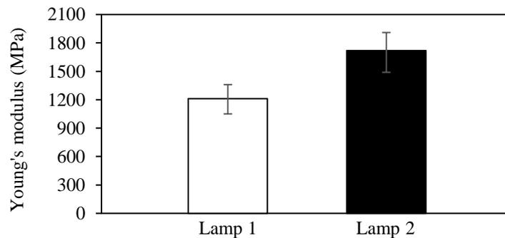
Figure 6: Young's modulus of high speed sintered parts
