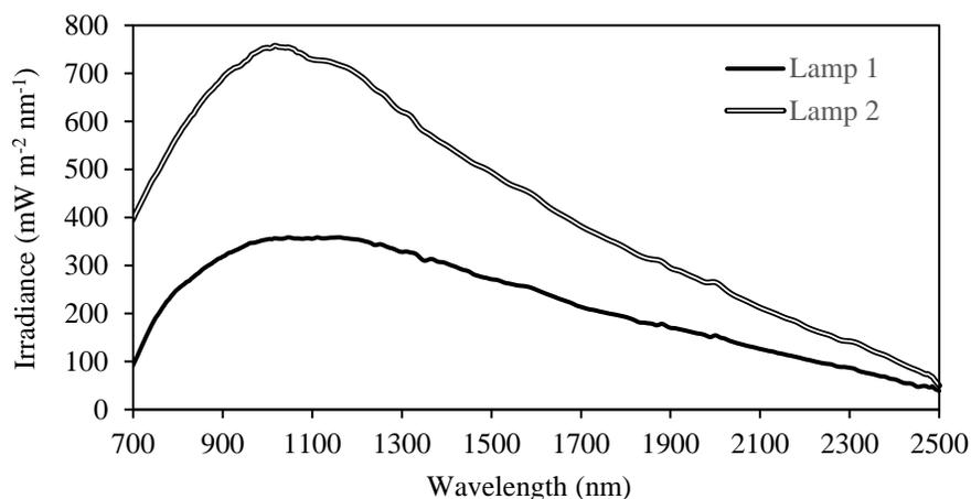
Figure 4: Spectral output of the infrared lamps
