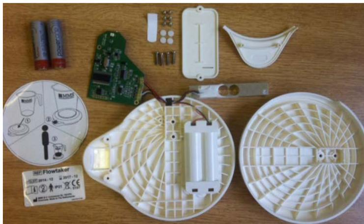
Figure 2 – Disassembled overview on main individual components
