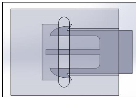
Figure 23. Fastened model of the reusable clip fastener
