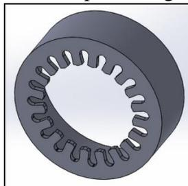
Figure 12. Modified guided icosafoil cap
