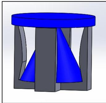
Figure 14. Fastened reusable claw with cone pin
