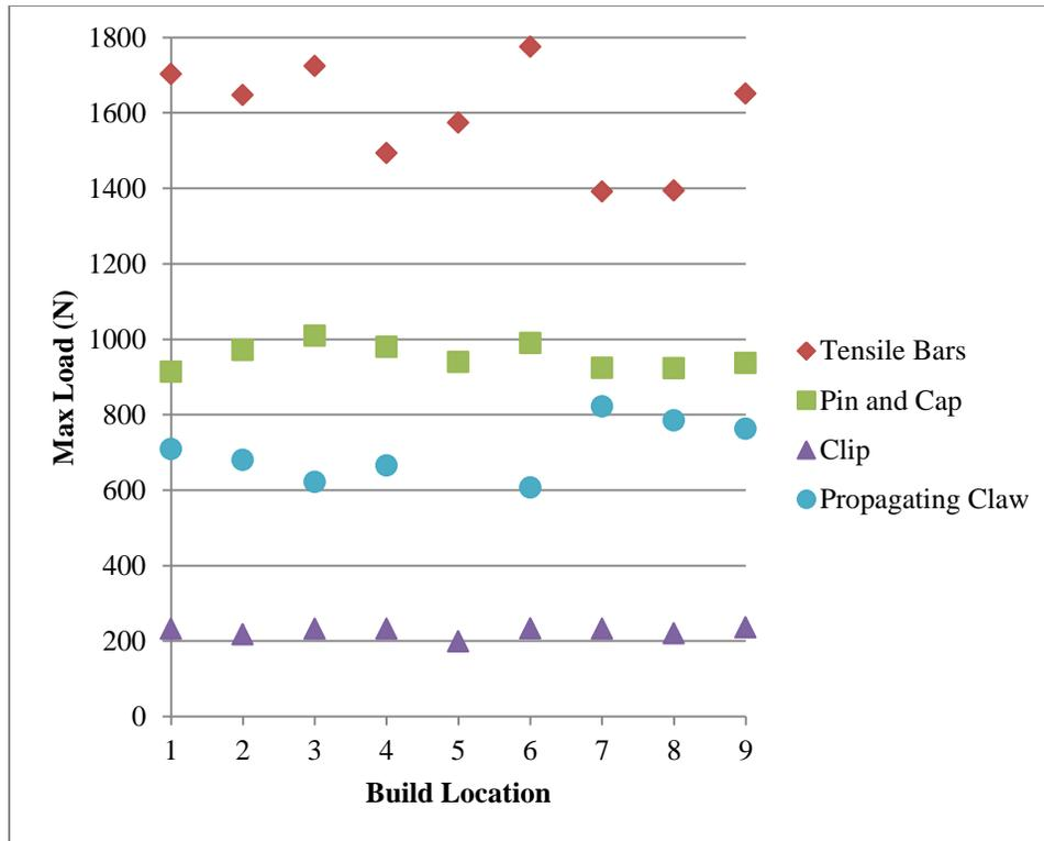
Figure 29. Tensile test results from the first build
