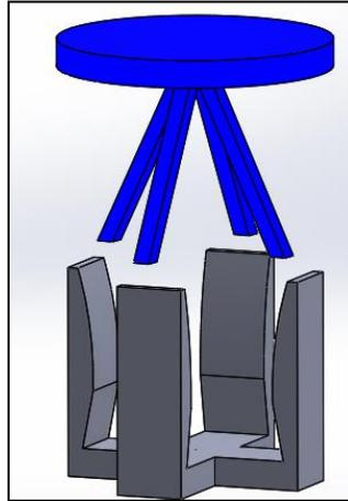
Figure 13. SolidWorks model of reusable claw fastener
