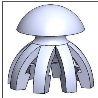
Figure 20. SolidWorks model of propagating claw fastener
