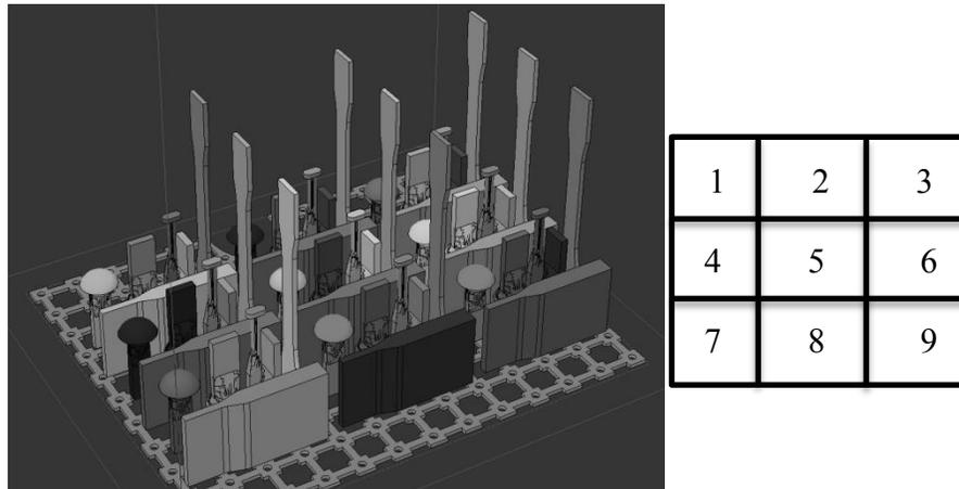
Figure 28. Build layout and numbering for variability testing
