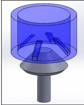
Figure 1. SolidWorks model of permanent cap fastener
