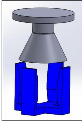
Figure 15. Reusable claw with modified pins
