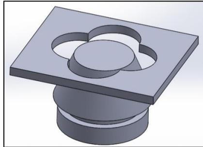
Figure 7. SolidWorks model of the permanent quatrefoil fastener
