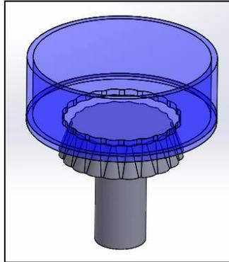
Figure 10. SolidWorks model of guided icosafoil fastener
