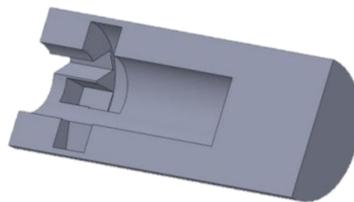
Figure 19. Section view of locking shaft fastener part 2
