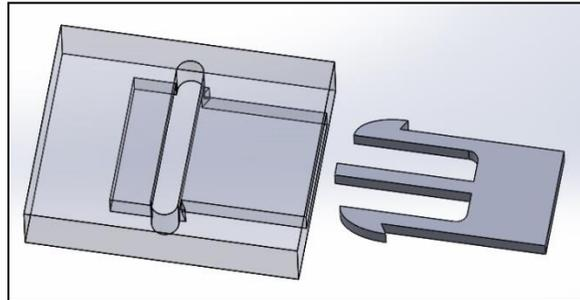
Figure 22. SolidWorks model of the reusable clip fastener
