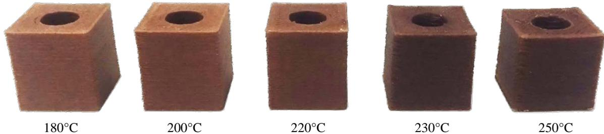
Figure 5: Cubes with different tones printed at differing temperatures with LAYWOO-D3 filament
