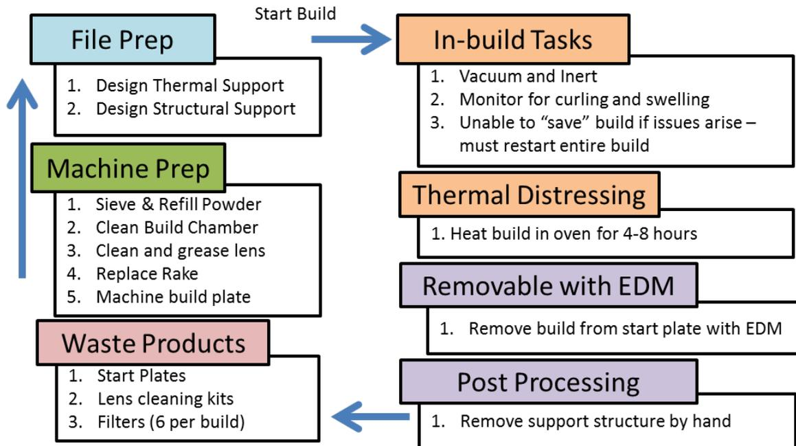
**Figure 2: Process cycle for LM**
