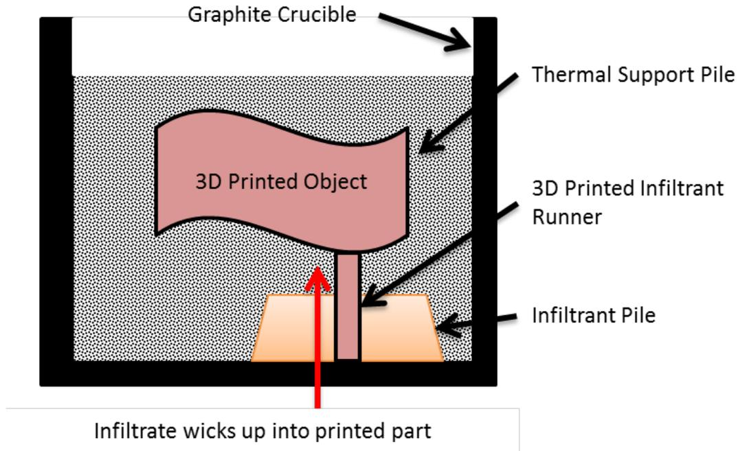
Figure 5: Setup configuration for the sintering and infiltration of I-3D printed green parts
