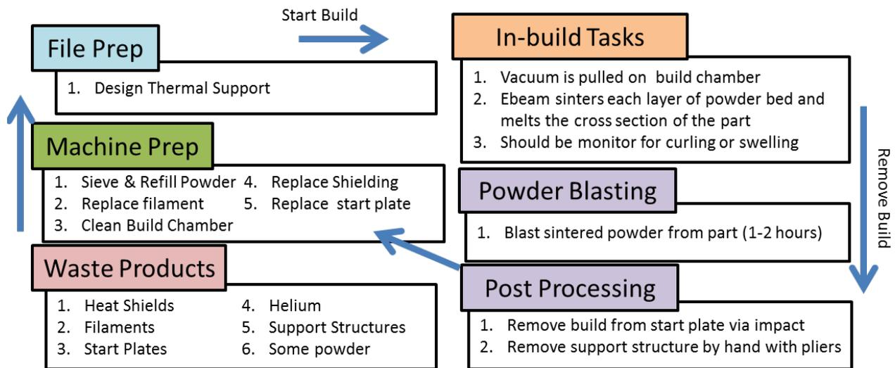
**Figure 3: Process cycle for operating EBM system**
