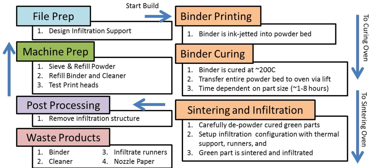
**Figure 4: Process cycle for binder jetting**
