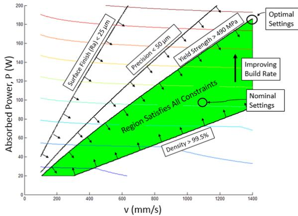
Figure 2: Case Study #1, showing objective contours of build rate overlaid on design constraint requirements
