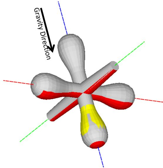
Figure 5. Type 1 surface (red), Type 2 surface (yellow), Type 3 surface (grey)
