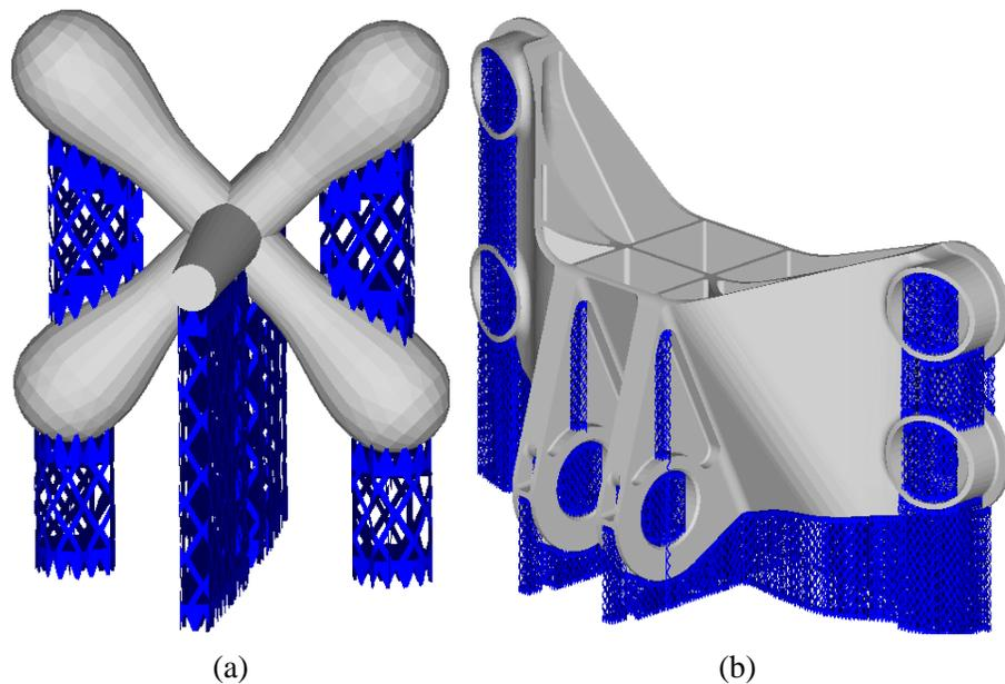
Figure 6. Optimized build orientation (a) Jack and (b) GE Engine Bracket
