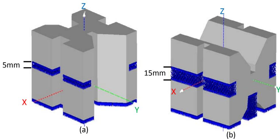
Figure 8. Two possible orientations with Z-height as priority
