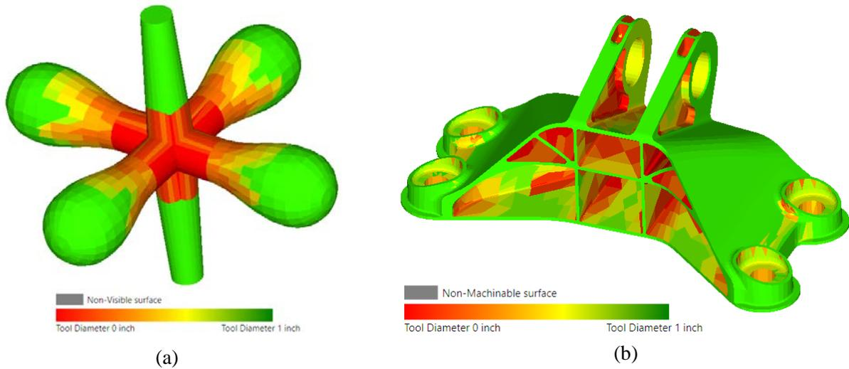
Figure 3. Tool accessibility maps (a) Jack and (b) GE Engine Bracket
