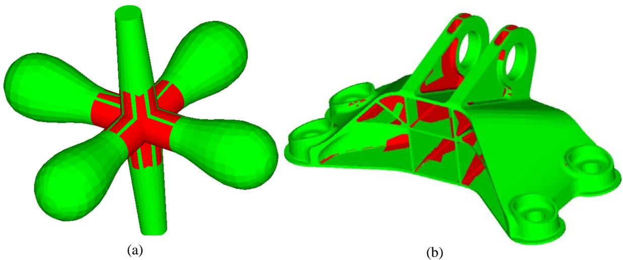
Figure 4. Non-accessible map (6.35 mm tool diameter) (a) Jack and (b) GE Engine Bracket
