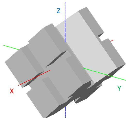
Figure 7. Best case for minimum support volume (Case 1)
