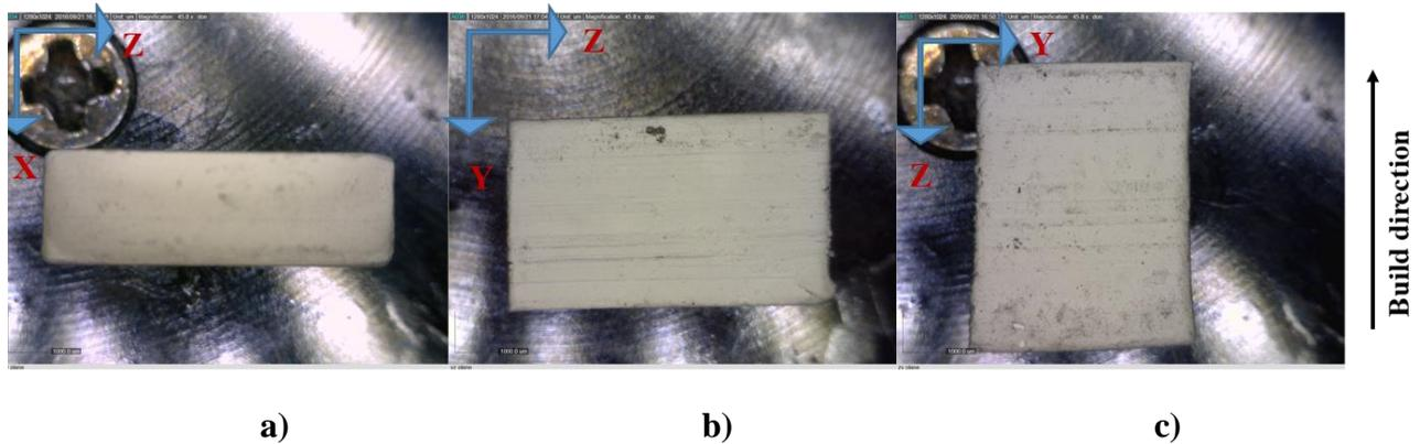
**Figure 6.** Layered profiles of sintered TCP parts with respect to build orientation: a) xy-plane (flat), b) yz-plane (edge) and c) zy-plane (vertical). Magnification: 46X
