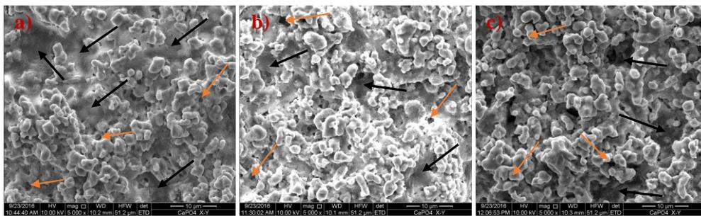
**Figure 4.** The bulk microstructure of TCP specimens fabricated in the **a)** x-y (Flat), **b)** y-z (Edge) and **c)** z-y (Vertical) build orientations. Black arrows denote large-scale voids beneath the fracture surface. Orange arrows denote smaller voids present at the specimen's surface. Magnification: 5000X
