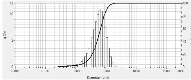
**Figure 5.** Particle size distribution of TCP powder feedstock used for printing. Q (%) represents percent frequency related to histogram data. Undersize (%) represents cumulative percentage of particles below the particle diameter.
