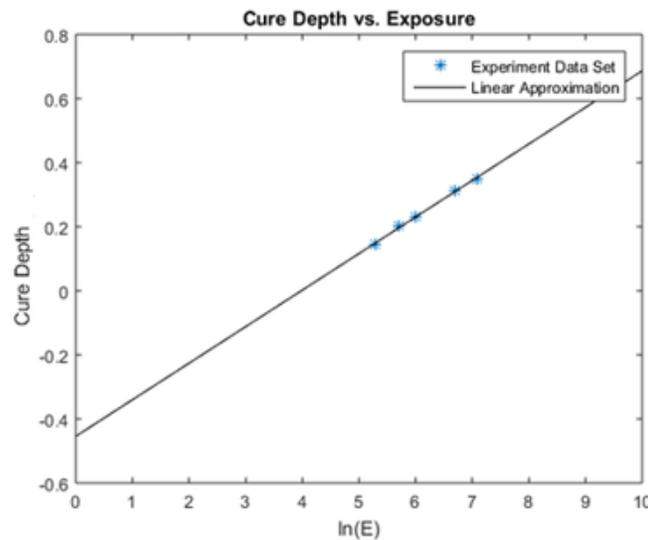
**Figure 3.** A semi-log plot of the working curve for TCP suspension. Energy exposure ( $\text{mJ}/\text{cm}^2$ ) and Cure depth ( $10^{-4}$  m) are in the x and y-axis respectively.
