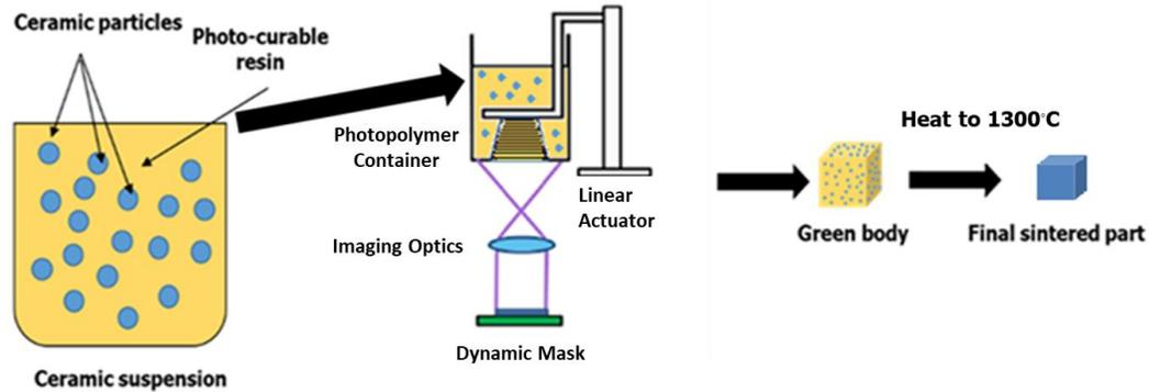
**Figure 1:** Schematic representation of ceramic suspension process for vat photopolymerization.
