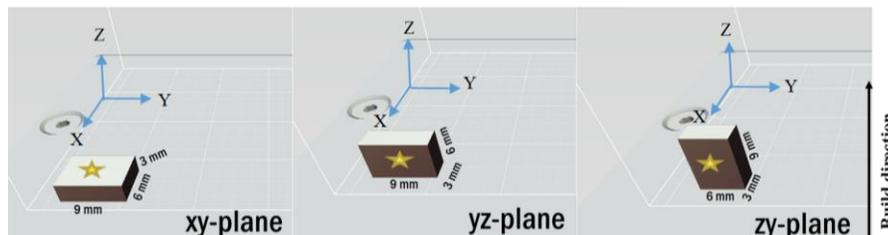
**Figure 2.** CAD designs of cuboids oriented on the build platform in the xy, yz, and zy-planes. The build direction occurs in the z-axis. \*Denotes the reference face that is parallel to the plane of interest in the cartesian coordinate system.
