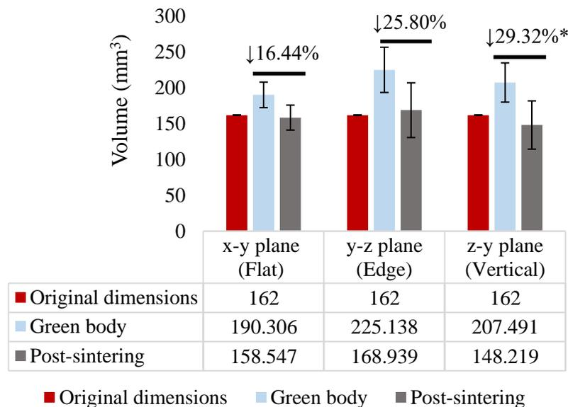
**Figure 7.** Volumetric shrinkages of TCP parts with respect to build orientation. (\*denotes statistical significance at  $p < 0.05$ )
