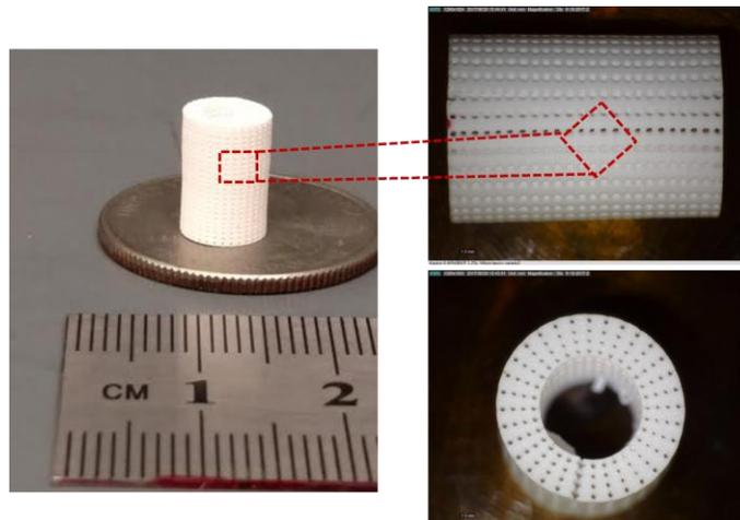
**Figure 9.** A sintered porous alumina bioceramic cylindrical scaffold under light microscopy. 30X Magnification
