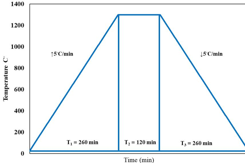
**Figure 3.** Sintering cycle of TCP specimens.
