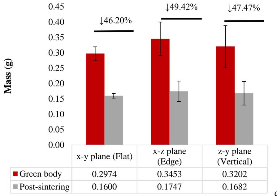
**Figure 8.** Mass loss in TCP cuboid specimens with respect to build orientation after sintering.
