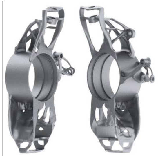
Figure 5: Example for bad geometry retransition by manual NURBS creation [RK15]
