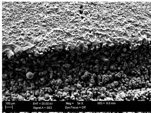
Figure 1. SEM image of a PBF/Ti-6Al-4V mini-channel adjacent to a machined surface.
