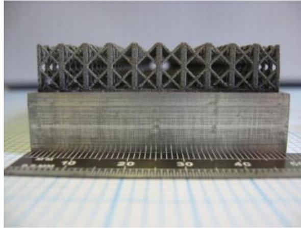
Figure 2. Lattice-structured heat sink fabricated via L-PBF [34]. *Used with permission.*
