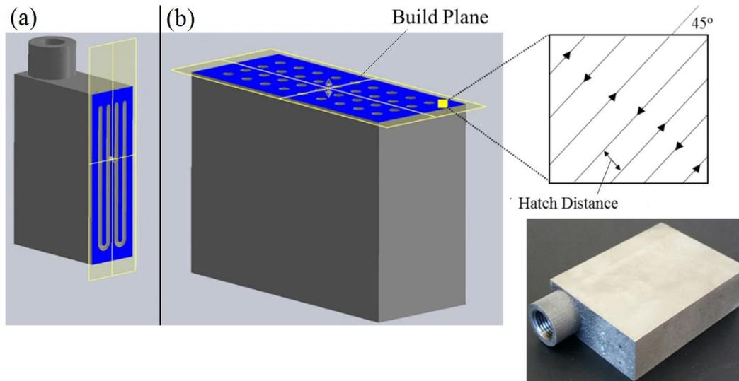
Fig. 3. The FP-OHP with build plane (a) shown relative to fill port and (b) relative to powder bed including the laser path directions and hatch distance. Photograph of finished Ti-6Al-4V also shown [8]. *Used with permission.*
