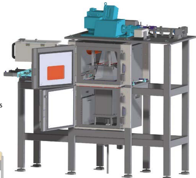
Figure 1: SLS test equipment for material qualification (Developed at Paderborn University in collaboration with the PROTIQ GmbH)
