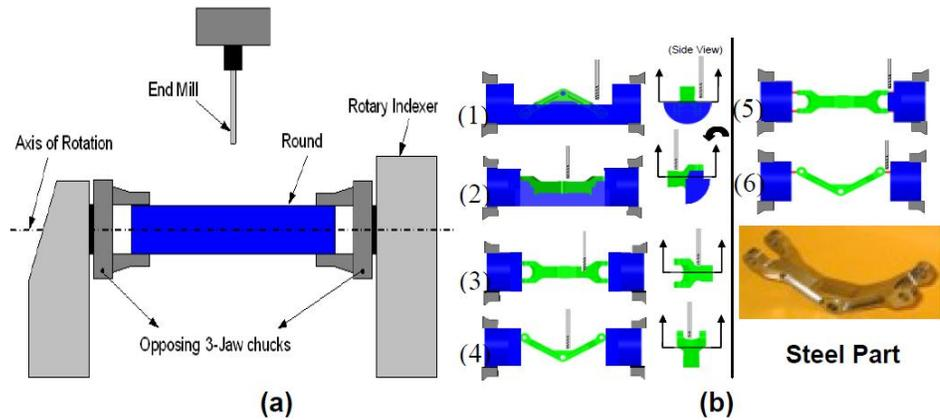
Figure 3: CNC-RP Process, (a) Rotary fixture setup; (b) Process sequence of steps (1- 6) to produce a steel component
