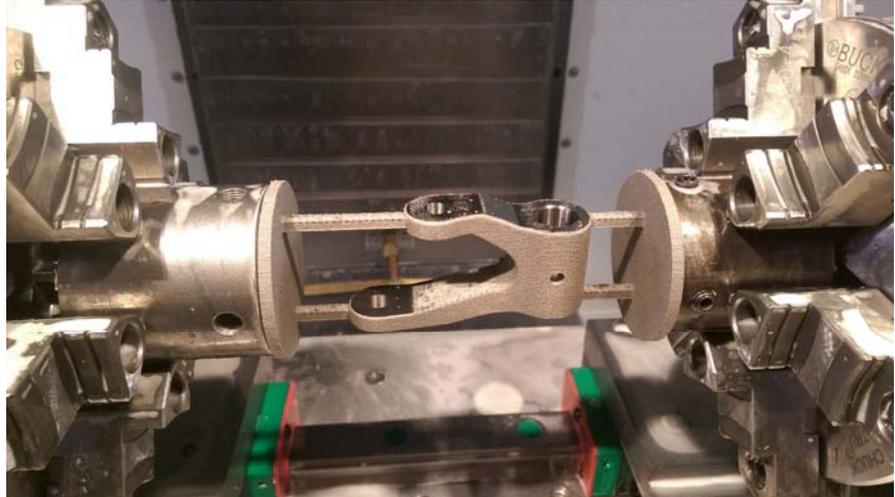
Figure 11: DASH processed part immediately after machining
