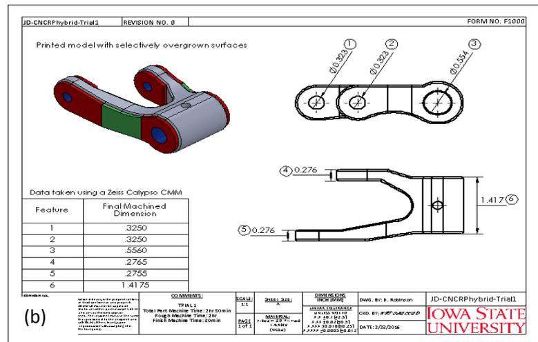
Figure 12: Titanium part sample; (a) progression across the process, and (b) CMM analysis data on nominal dimensions
