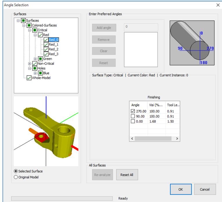
Figure 9: CNC-RP toolpath planning interface
