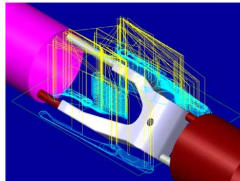
Figure 10: Roughing toolpath calculation
