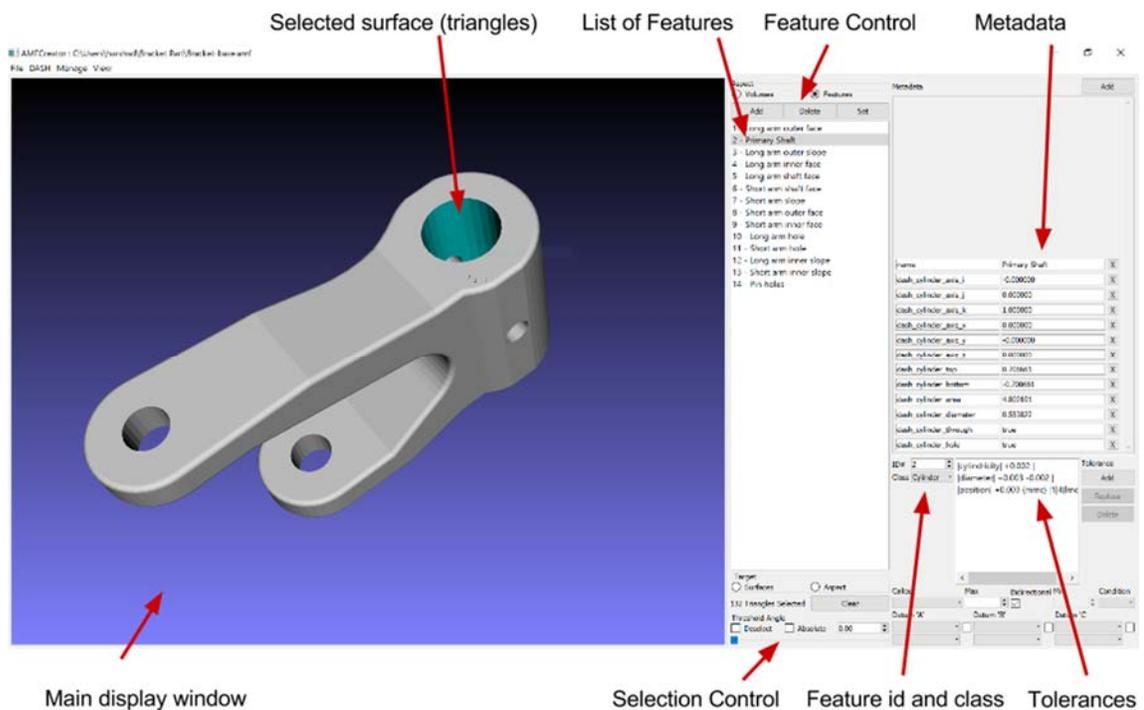
Figure 2: AMFCreator software interface
