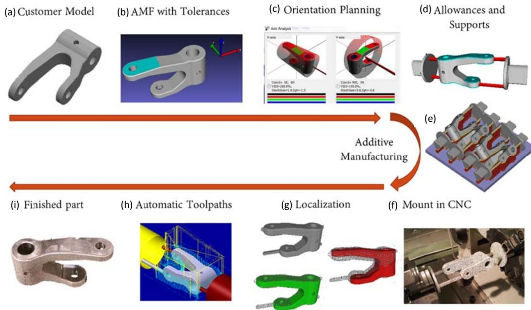
Figure1: DASH Process Flow; (a) Customer model input, (b) AMF model creation with critical features identified, (c) Machining setup orientation planning, (d), Addition of machining allowance and sacrificial fixture supports, (e) Metal AM processing, (f) clamping in CNC mill, (g) scanning and part localization, (h) automated toolpath generation, (i) finished part after support removal
