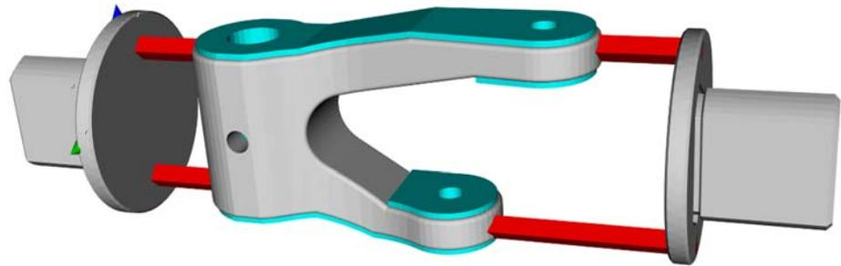
Figure 6: Part model in AMFCreator, with sacrificial supports, fixture clamping elements, and machining allowance on critical surfaces
