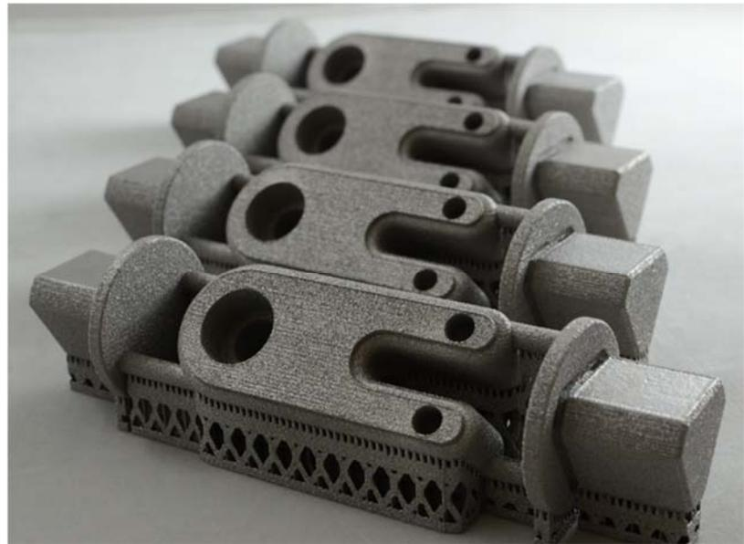
Figure 7: Part, AM supports, and Sacrificial supports to fixture clamping elements after powder bed metal printing
