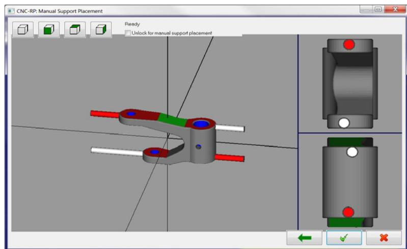
Figure 5: Sacrificial support placement interface
