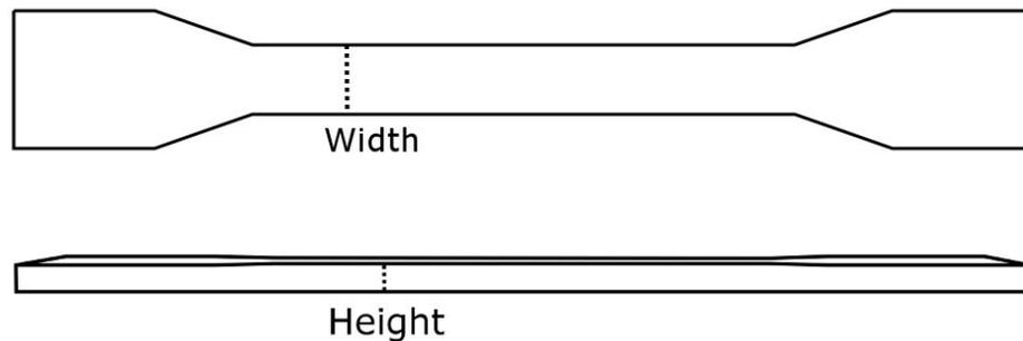
Figure 2. A tensile bar and how the width and height measurements are taken shown schematically.
