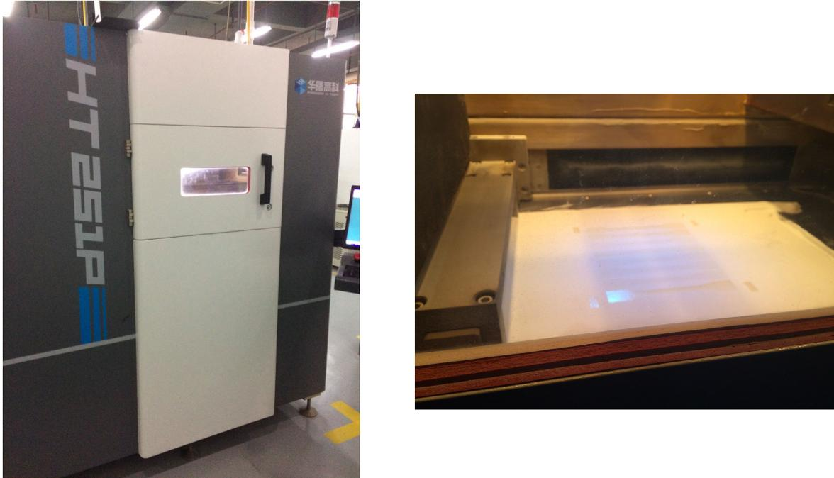
Figure 1. (Left) Farsoon HT251P SLS-machine used for the experiments. (Right) An image captured during the scanning process.
