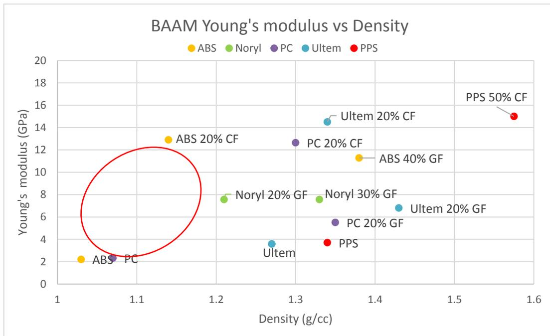
**Figure 1.** BAAM specific material property space map. The area circled in red identifies potentially accessible region with functionally graded materials
