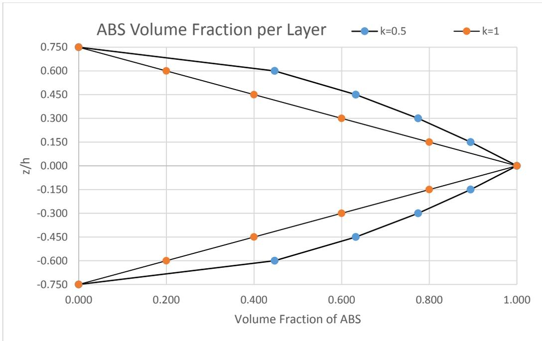
**Figure 3.** Volume percent of ABS in the FGM sandwich panel at each layer.  $Z/h$  represents distance from the neutral axis
