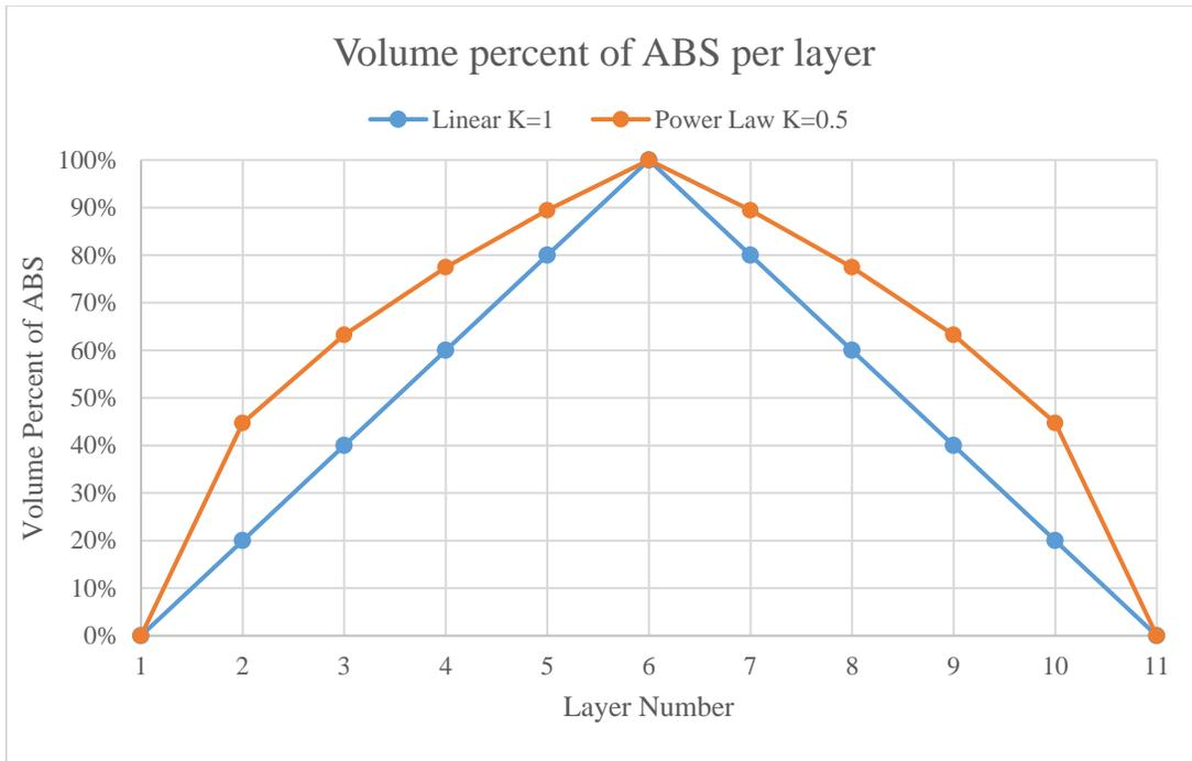
**Figure 4.** Graph representing the volume fraction in percent of ABS in each layer for both the Linear and Power Law variations
