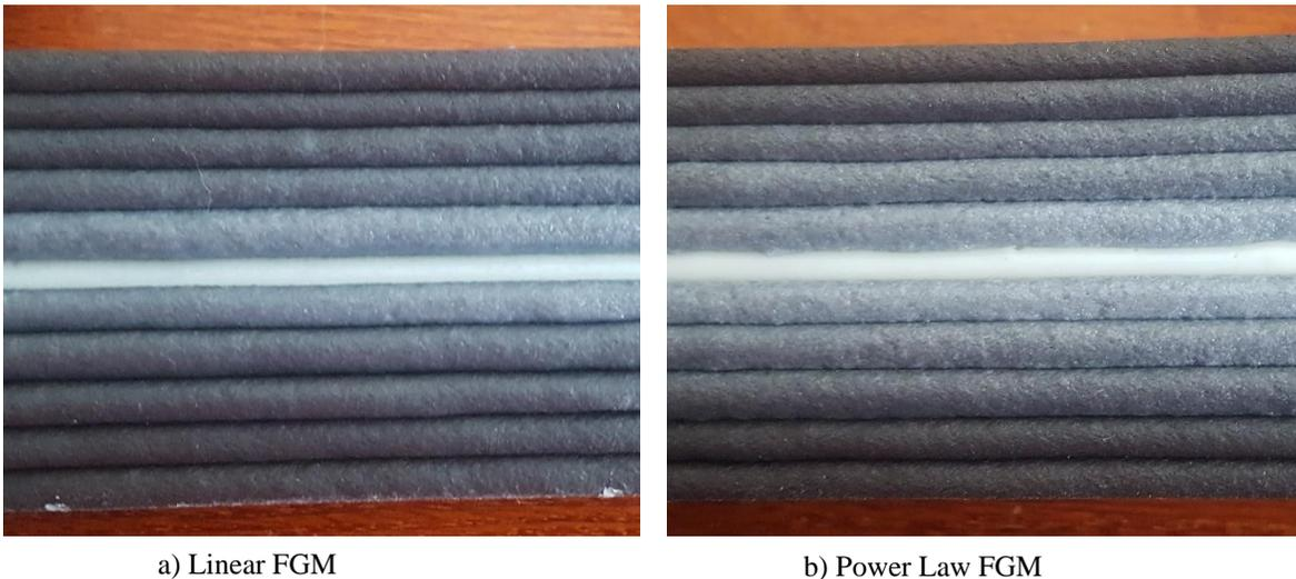
**Figure 6.** Pictures of printed sandwich panel beams with functionally graded core
