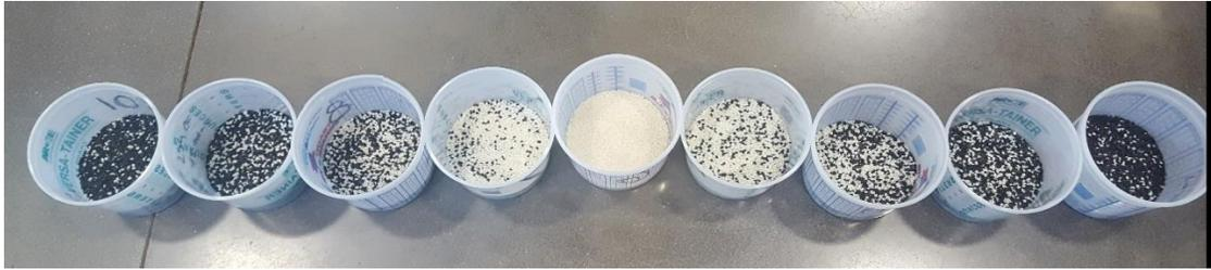
**Figure 5.** Picture of the pre-mixed material for each layer. The white pellets are ABS, and the black pellets are CF-ABS
