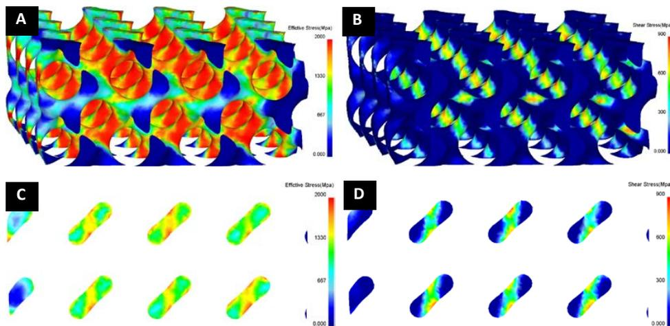
Fig.3 Stress distribution of the Gyriod cellular structure at 5% overall deformation: (A) Von Mises effective stress distribution,(B) 45°shear stress distribution,(C) Von Mises effective stress distribution on the vertical plane, and(D) 45°shear stress distribution on the vertical plane.
