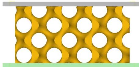
Fig 2 FEA model of the uniaxial compression test
