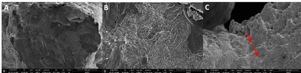
Fig.5 Fracture and surface morphologies of the test sample after 30% deformation: (A) Smooth river and shell patterns, (B) Small and irregular dimples, and(C) Surface
