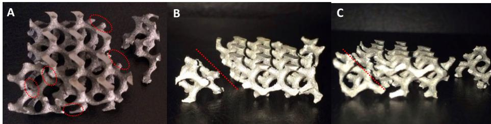
Fig.4 Observations from different perspectives after 30% deformation: (A) Fracture positions observed from the top view, (B) Fracture zone direction observed from the front view, and(C) Fracture zone direction observed from the back view.
