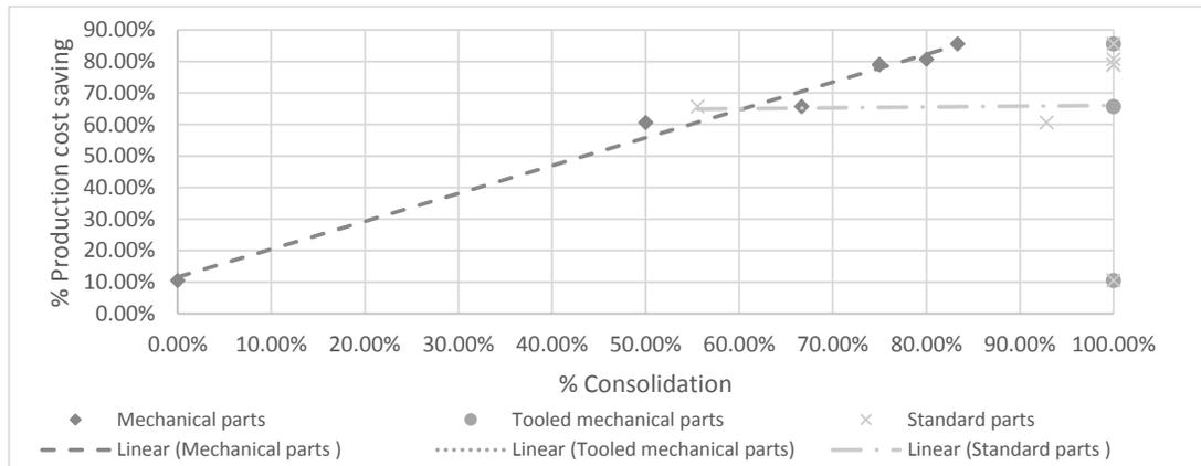
Figure 6 Consolidation against production cost saving for the mechanical parts, tooled mechanical parts, and standard parts
