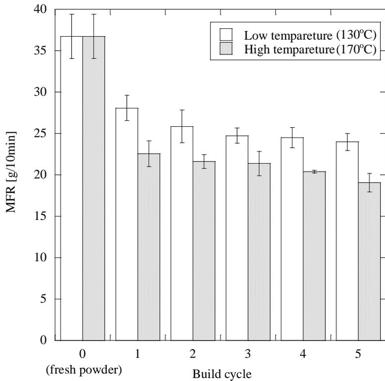
Figure 6. MFR of unmetled powder in each build cycles
