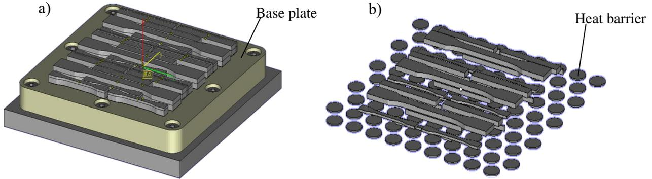
Figure 2. Build layout a) low temperature process b) high temperature process
