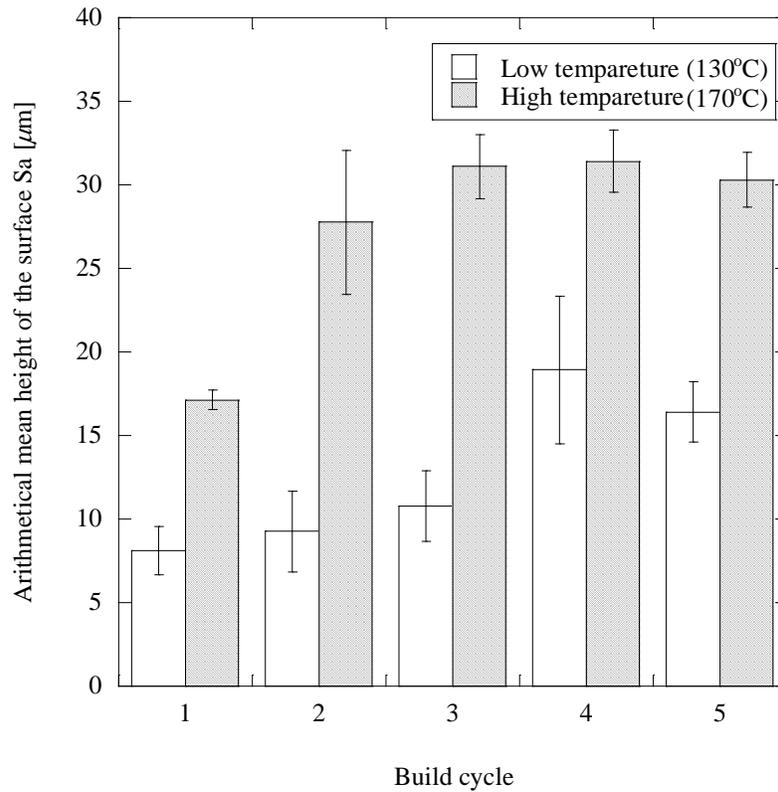
Figure 5. Arithmetic mean height  $S_a$  of each build cycles
