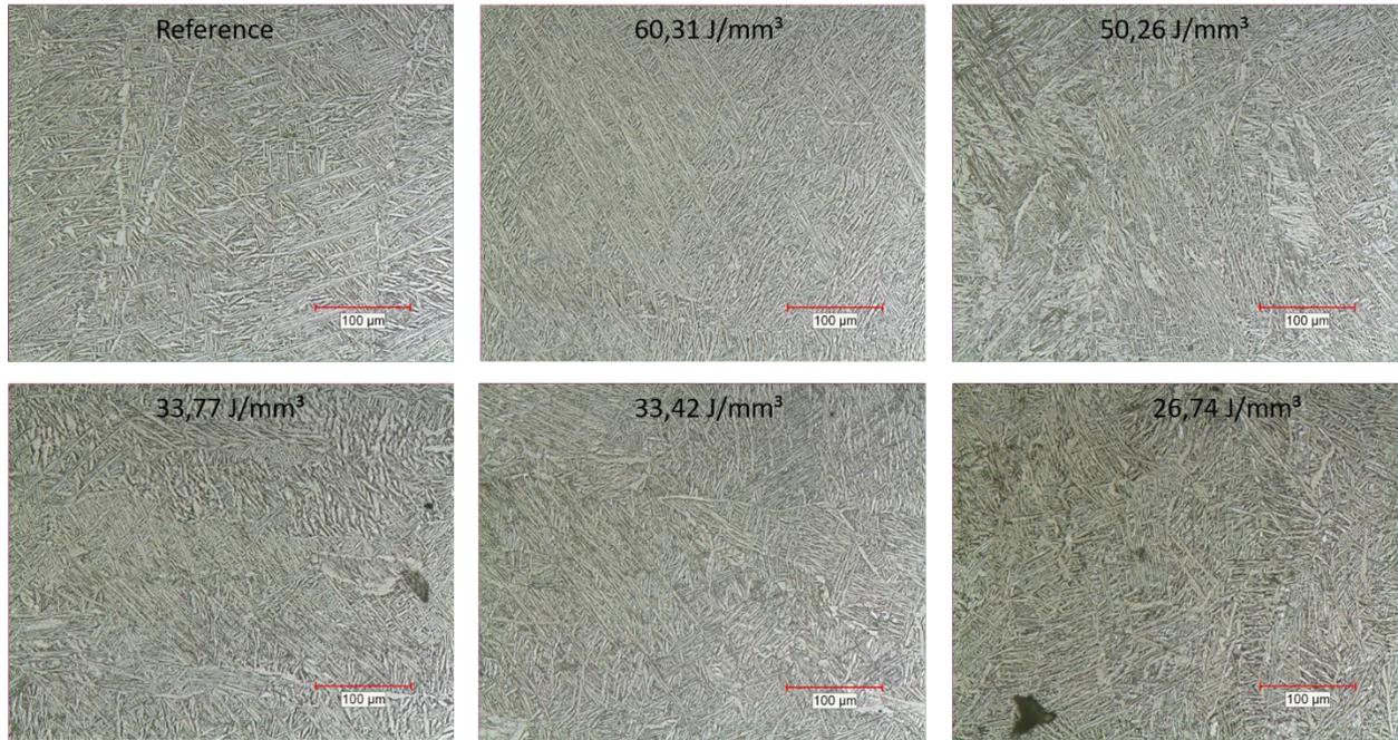
*Figure 4 – Microstructure of Ti6Al4V specimens with different parameter sets*
