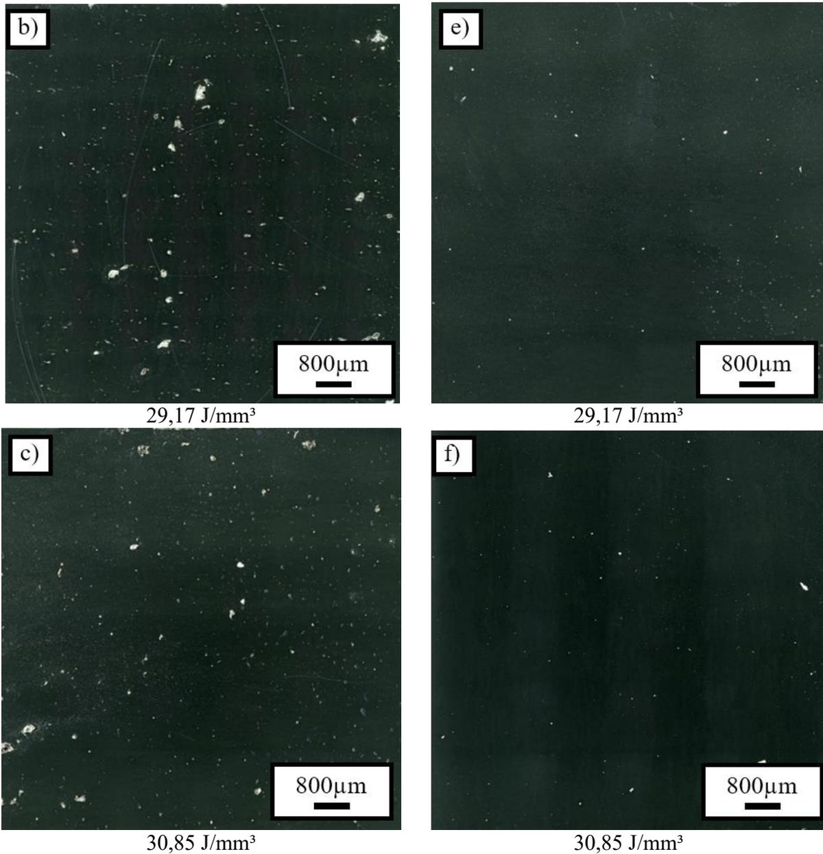
Figure 2 - Dark field optical images displaying cross sections of the SLM processed specimens in the as-built condition (a)-(c) as well as the HIP-condition (d)-(f).
