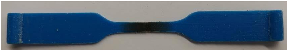
Figure 9. Voxel printed specimens with true material gradients
