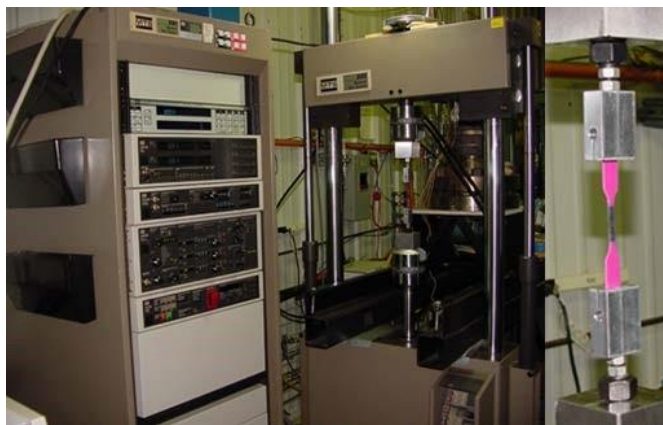
Figure 10. The MTS 880 Servohydraulic Material Testing System (left) and the non-compression grips and a sample specimen (right)
