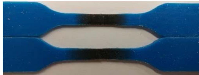
Figure 6. Specimens showing true material gradients: min-length (top) and max-length (bottom)
