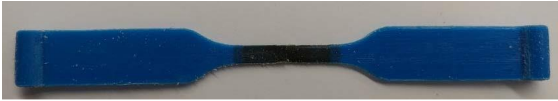
Figure 8. Printed specimens with discrete material gradients
