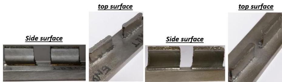
(a) 1.9-LED machined surfaces (b) 1.3-LED machined surfaces
