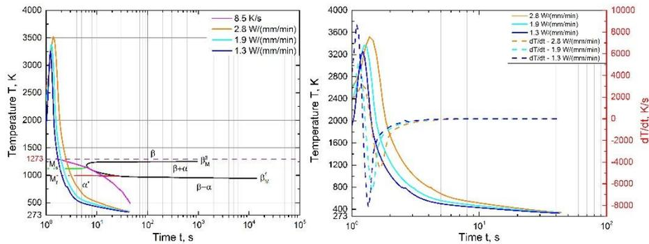
(c) cooling curves with CCT diagram
