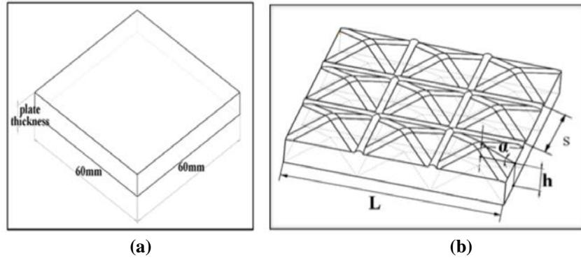
**Figure 2** Overview of specimen structure (a) planar plate, (b) pyramid structured plate:  $\alpha$ - pyramid angle,  $h$ -plate thickness,  $s$ -pyramid element length.
