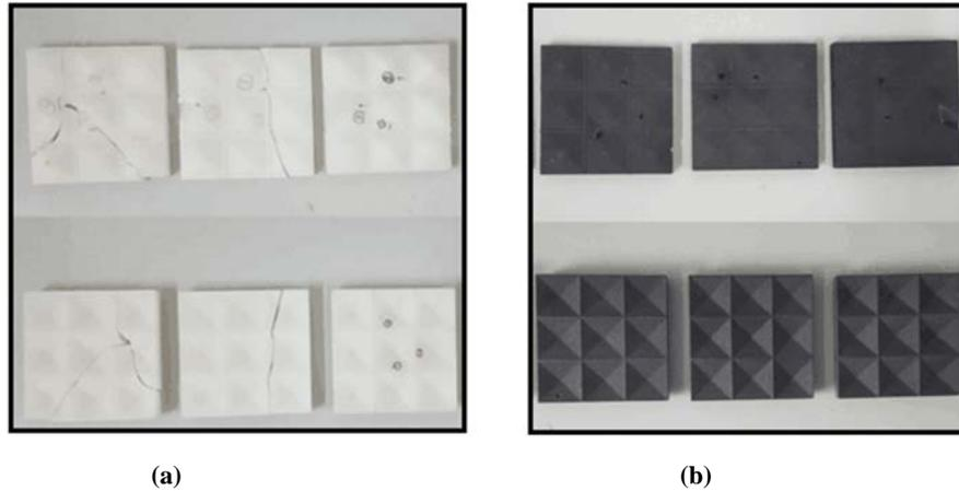
**Figure 5** Experimental test results from the structured laser sintered PA 3200 and PA/CF, with tilt angle of  $20^\circ$ , plate thicknesses of 6,5 7, 7.5 mm from left to the right, first row: front view, second row: back view, (a) laser sintered PA 3200, (b) laser sintered PA/CF
