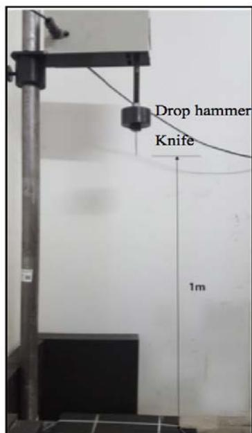
**Figure 1. Stab resistance test platform**
