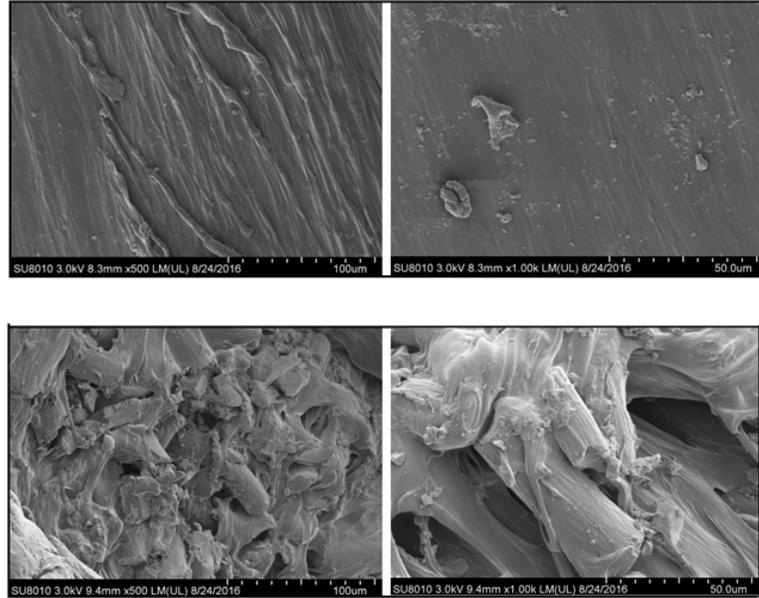
**Figure 6:** SEM images of the cross section of the structured specimen with a thickness of 7 mm and tilt angle of 20°, (a) laser sintered PA 3200 (top row), (b) laser sintered PA/CF (bottom row)
