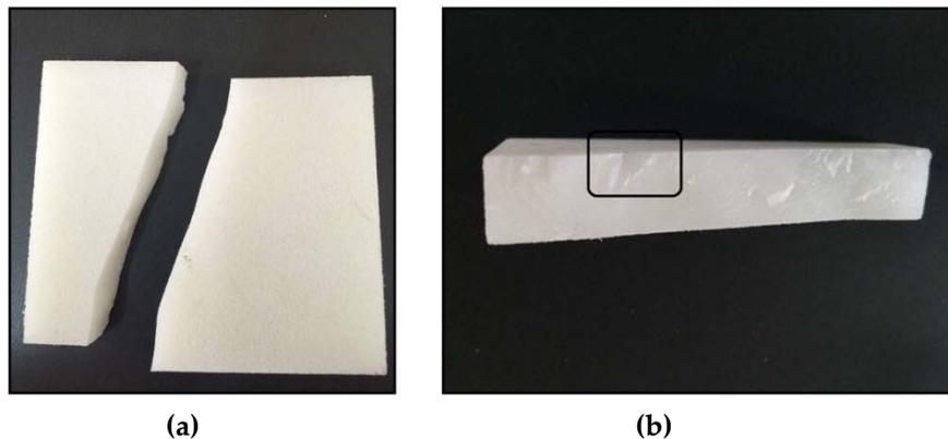
**Figure 4** 8-mm-thick laser sintered PA 3200 after the stab resistance experiments (a) front view of the broken sample, (b) cross section view of the broken sample
