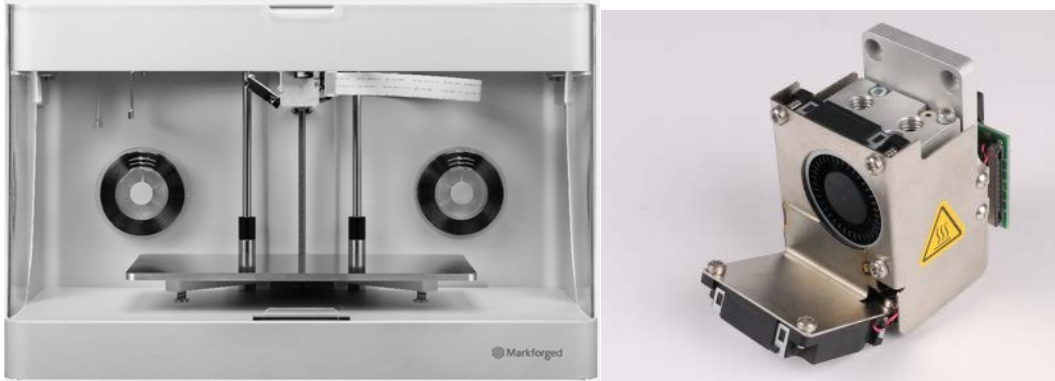
Fig. 1: The CFF AM Equipment (MarkForged MarkOne) and the Print Head with 2 nozzles
