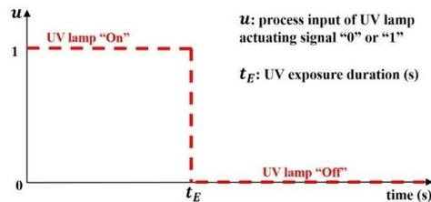
Fig. 2. On-Off control input in the ECPL process
