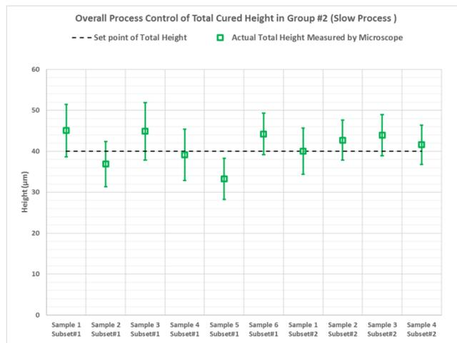
Fig. 8. Overall process control results for the parts cured in the real-time measurement and control experiments Group #2
