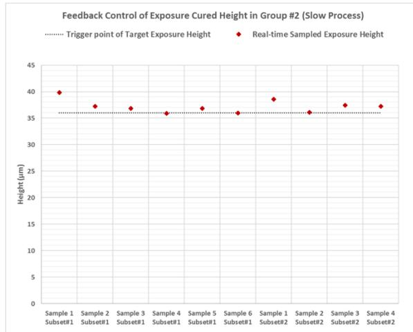
Fig. 6. Real-time feedback control results for exposure height in the real-time measurement and control experiments Group #2
