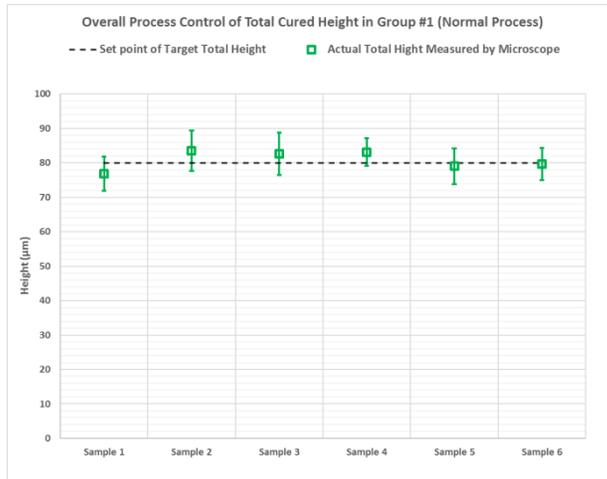
Fig. 7. Overall process control results for the parts cured in the real-time measurement and control experiments Group #1
