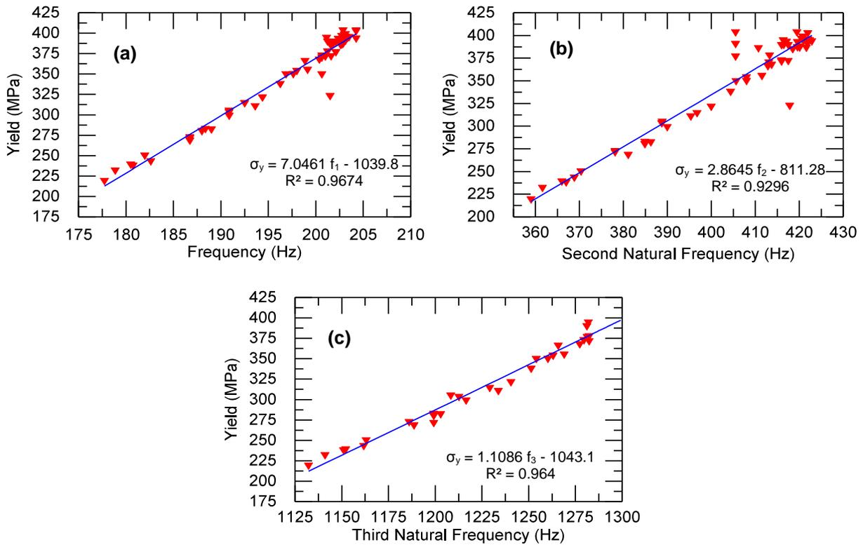
Fig. 7. Yield strength versus natural frequencies of (a) 1<sup>st</sup>, (b) 2<sup>nd</sup>, and (c) 3<sup>rd</sup> modes.
