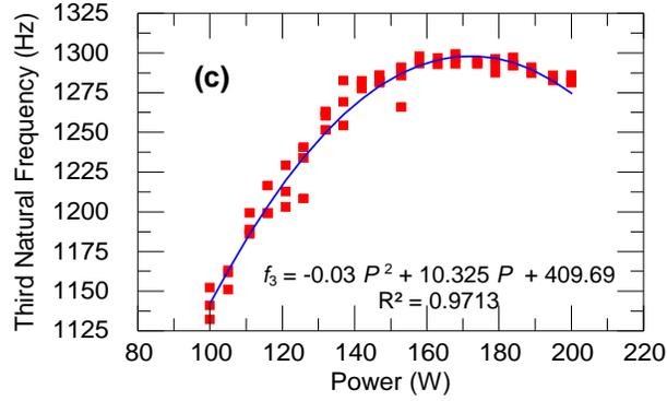
Fig. 6: Part Natural Frequency versus applied power for (a) 1<sup>st</sup>, (b) 2<sup>nd</sup> and (c) 3<sup>rd</sup> modes.
