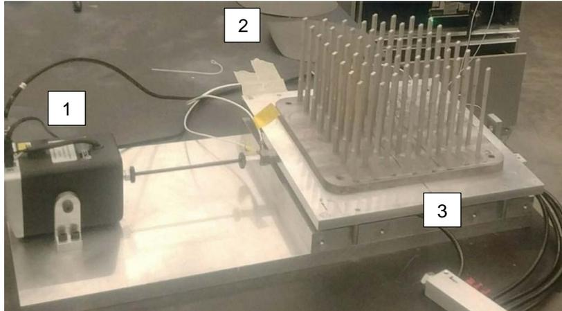
Fig. 2: Experimental setup of the 60 tensile specimens on a single plate. (LDV not shown).
