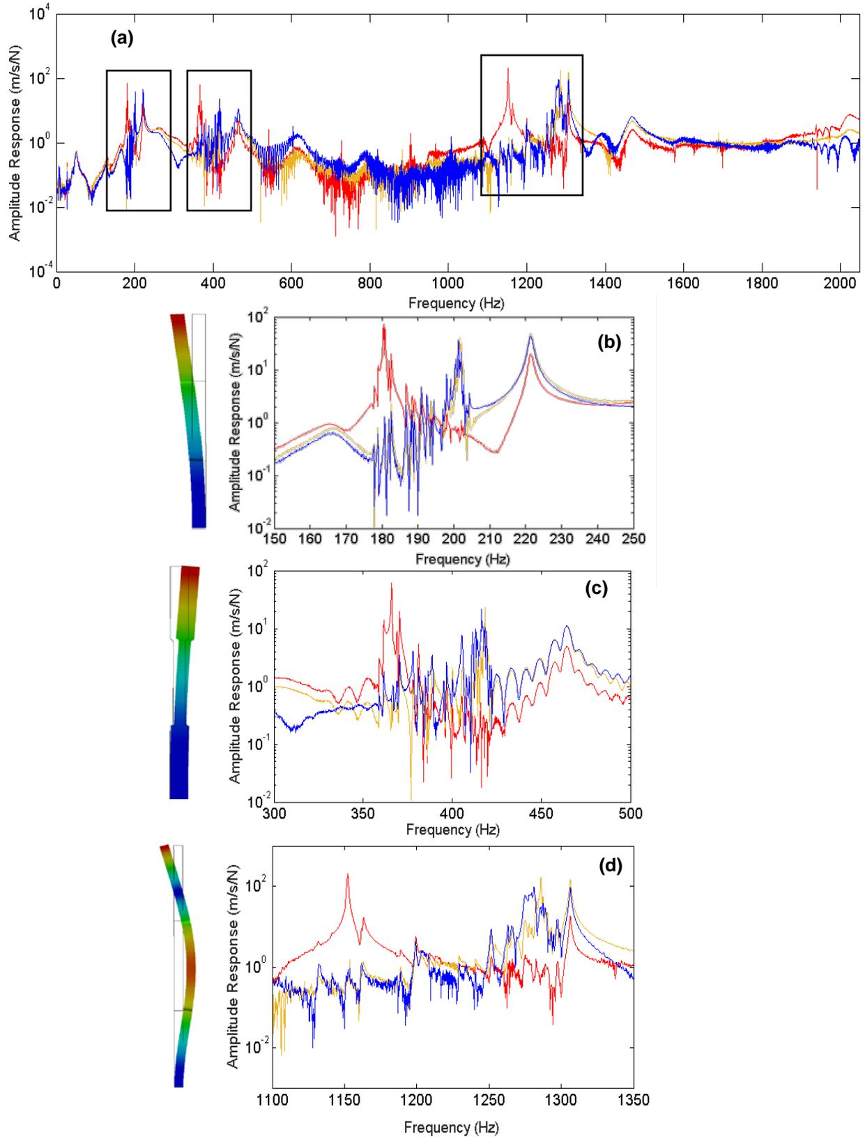
Fig. 3. Representative FRFs for various powers; red: 100 W (5,3), orange 147 W (6,5), blue: 200 W (2,2). (a) Full spectrum, (b) 1st mode, (c): 2<sup>nd</sup> mode and (d) 3<sup>rd</sup> mode.
