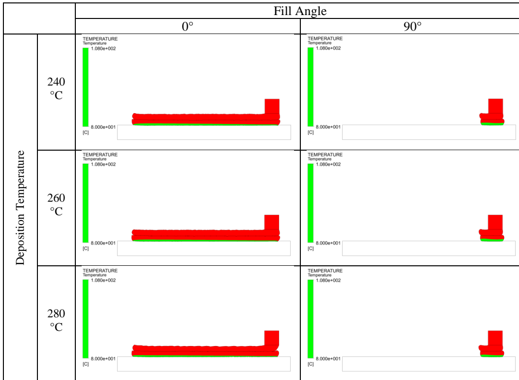
Figure 10. Temperature distributions from process simulation models with various fill angles and deposition temperatures
