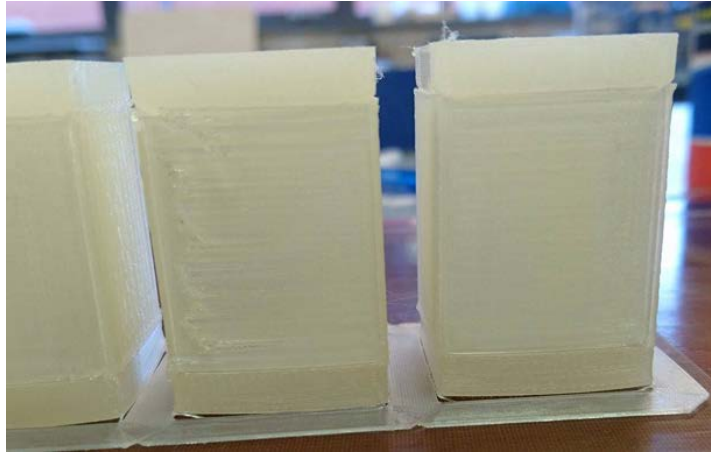
Figure 7: Thermal distortion in original Set 1 specimens.
