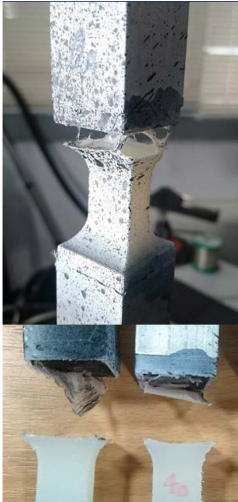
Figure 10: The ductile fracture interface of Set 1 specimens
