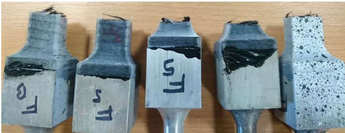
Figure 12: The fracture interface of Set 4 specimens. Torn fibres suggest prominent role of CF in providing tensile strength
