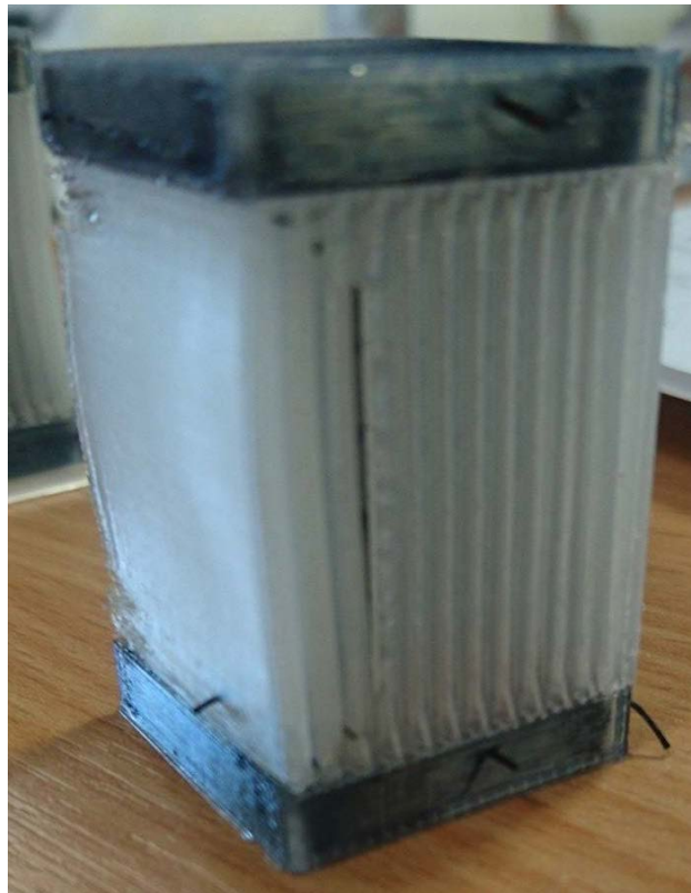
Figure 9: Set 4 specimen with CF splinters
