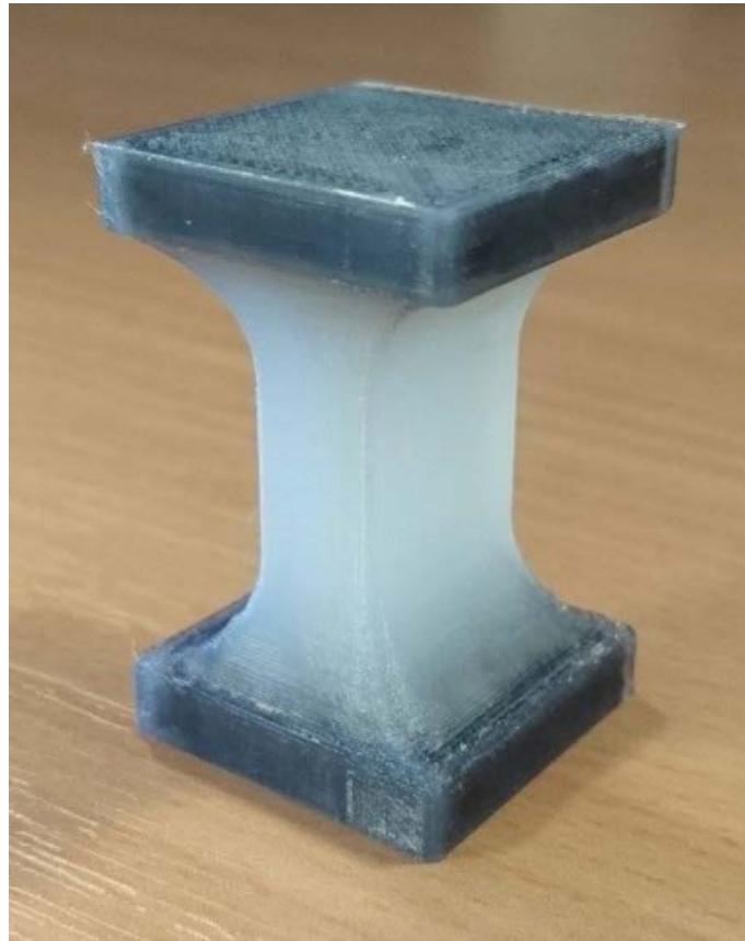
Figure 8: Set 1 (0% carbon fibre) specimen with reinforced bases.
