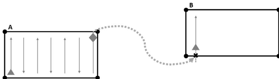
Figure 7. Illustration of a jump vector (dotted line) from layer part A to layer part B. The black dots indicate the starts and ends of the mark vectors representing the contour. The grey arrows indicate the hatching lines. The grey rectangle/square represent the start/end of the first/last hatching line. The square is also the take-off point of the jump vector. The end point of the jump vector is the black cross on the contour of layer part B.
