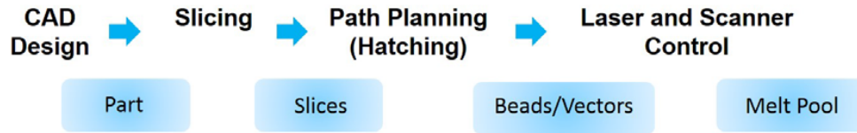
Figure 1. The workflow of process planning for the powder-bed based layered manufacturing process.
