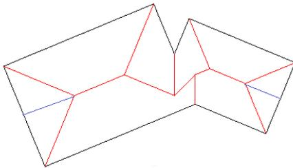
Figure 6. Straight skeleton of polygon without holes
