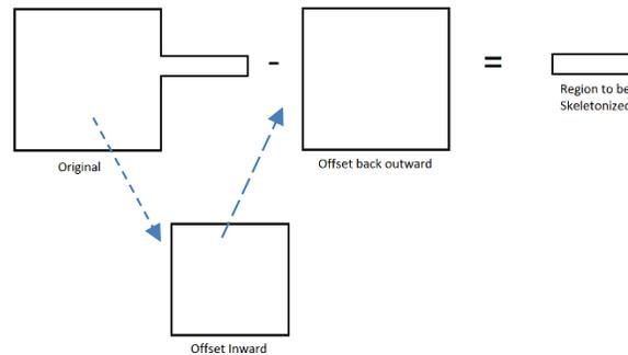
Figure 4. Void detection
