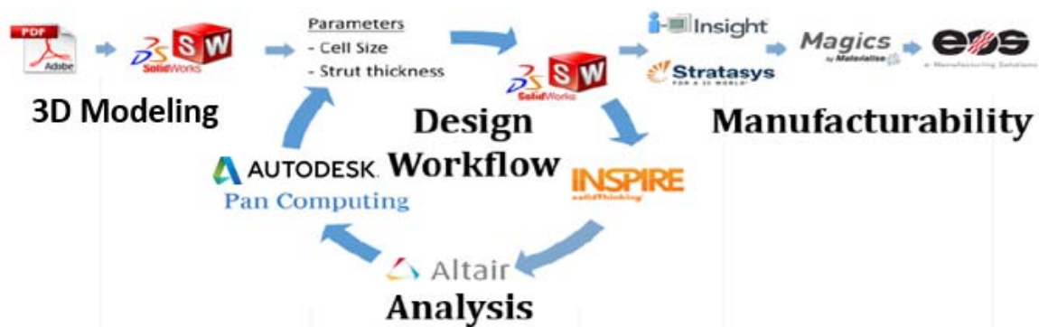
Figure 2: Illustration of software workflow from preparing 3D model of lattice structures to metal fabrication of final parts
